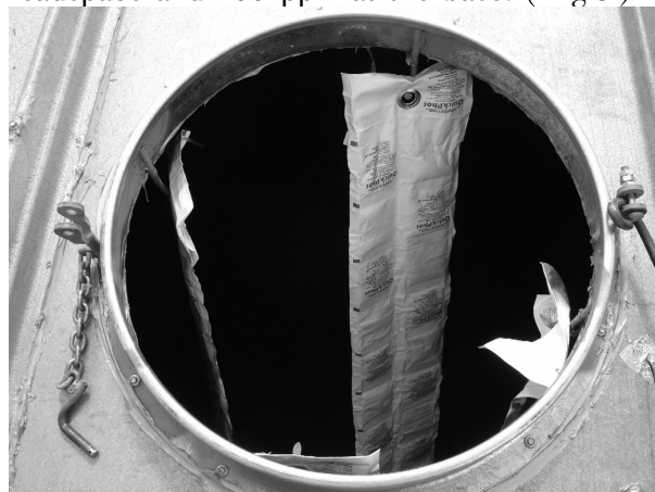
Fig. 4 Phosphine blankets suspended in fumigation hatch
